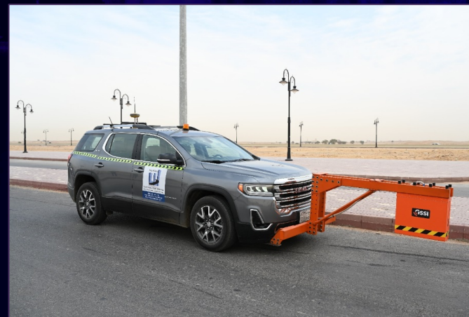
Ground Penetrating Radar (GPR)
